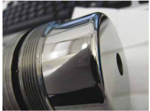
Chemically nickel plated mold insert, high-gloss polished (Photo: NovoPlan)
