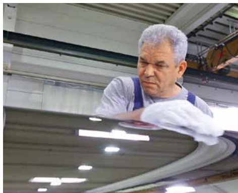
Roll: hard chrome coated and mechanically polished to high gloss (Photo: LKS)
