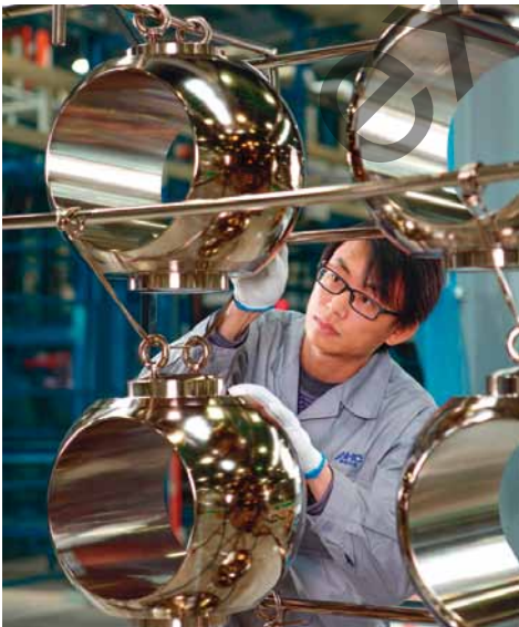
Shut-off ball valve, chemical deposited with nickel (Source: AHC)
